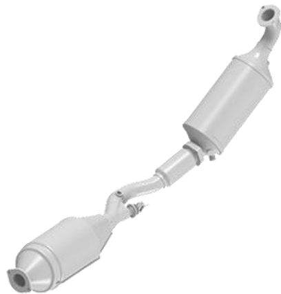
Hot end of exhaust system
